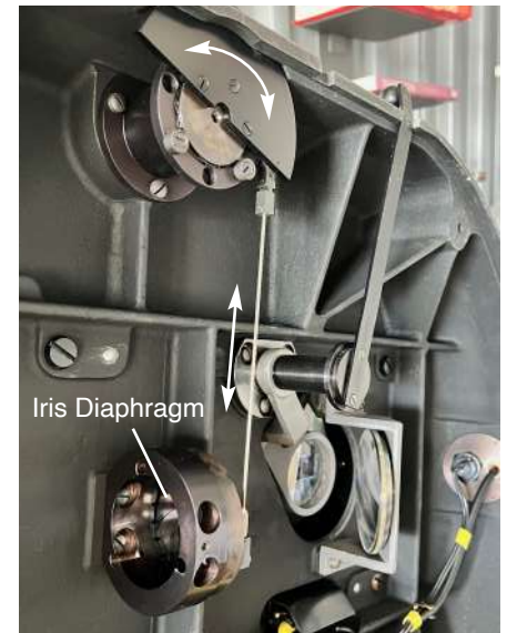
This dial controls the iris diaphragm via a linking rod (below).
