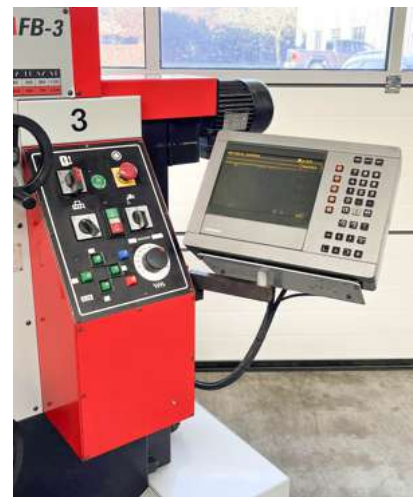
Power feed controls/DRO
