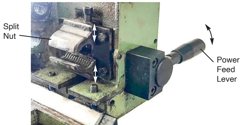
Cross slide split nut to engage/disengage to the lead screw activated by thread cutting lever
