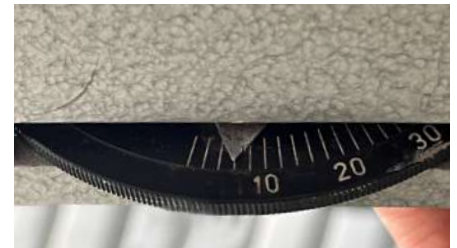
This dial controls the iris diaphragm via a linking rod (below).
