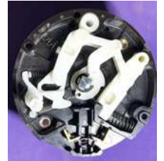
Inside Power Switch
