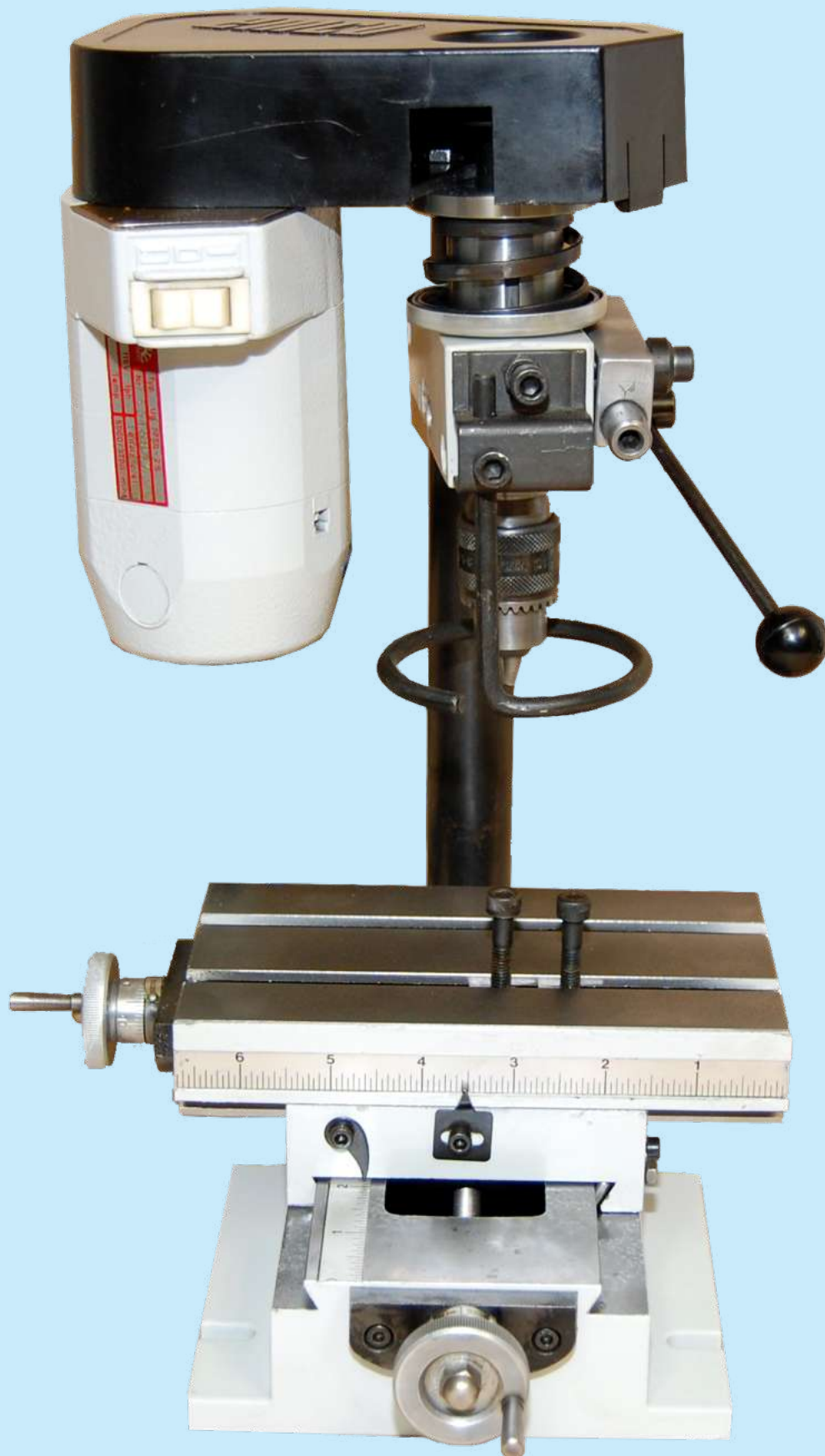
The precision hobbyist's machine. The legendary Unimat 3 on its optional X-Y milling table is a versatile table top machining center with numerous accessories for dividing, gear cutting, milling, drilling, and fly cutting operations. Over half a million Unimats 3's was sold world wide for their versatility, precision, and affordability.
