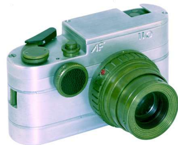
AF 110 camera 1981, built entirely with Unimat 3 When Dr. Ogura saw it, he said out loud: "Auto Focus!"
