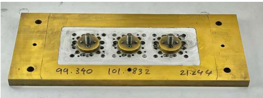
An interchangeable sub plate specially made for Optoform 50 mounts
