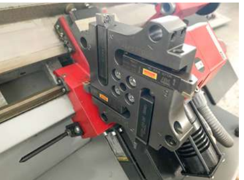
The automatic turret of Concept Turn 55 can carry 8 tools. Automatic turret is specially necessary for CNC lathes for high tolerance machining.
