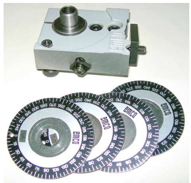
Unimat's dividing head also helped making many of Optoform's pieces. This is a compact, and versatile dividing head (compatible with Emco chucks with 14 mm thread) that can be utilized to fabricate small parts.
