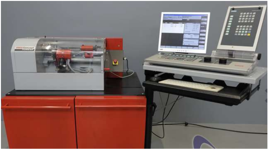
Concept Turnl 60 with faster feed rate, and more powerful motor with slant bed similar to production machines.
