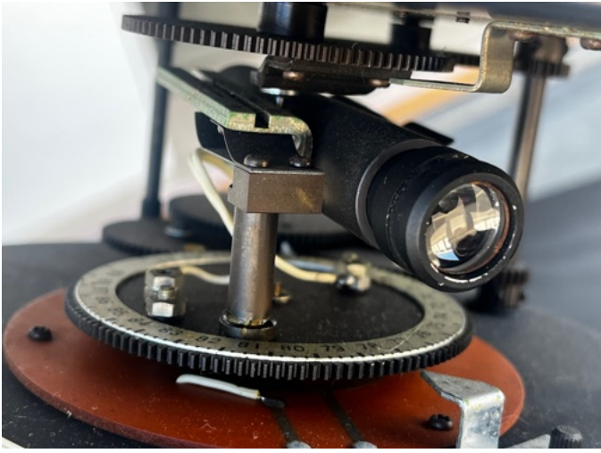
Right, the tilted Mercury orbit drive gear rotates back and forth because it is in the inner planets of the solar system. Mercury's movement as it moves across the sky is the most noticeable object in the planetarium.
