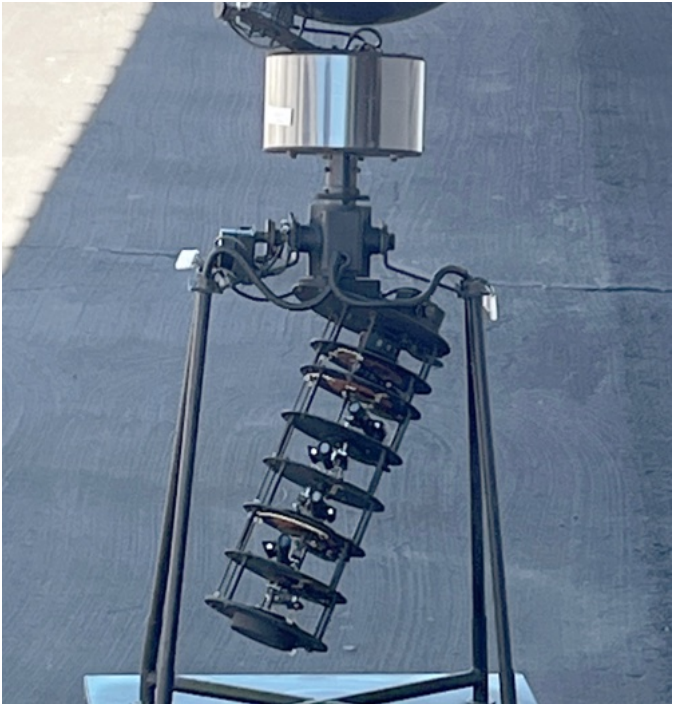
The electrical wiring of planetariums are challenging because it should be able to rotate 360 degrees on each axis. Some contacts like the central filament are powered by a brush + conductive disk method, similar to electric motor armatures.
