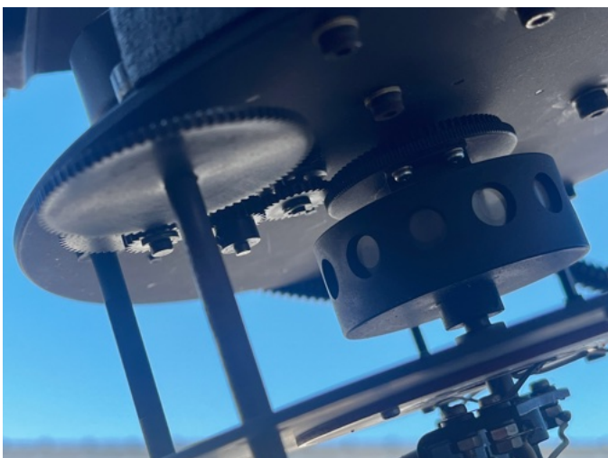
More details of the planetary, and lunar phase control gear train show the rotating control shaft, and how it drives the rotation of each planet across the sky. Watching Mercury is the most noticeable object in planetarium skies: Because it is in an inner orbit around the sun, it travels back, and forth instead of a continuous passage across the sky.
