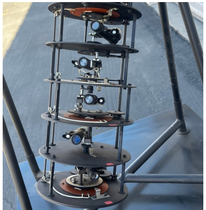
More detail of the graduated Meridian line projection cylinder (left), and labeled planetary discs from bottom to top: Saturn, Jupiter, Mars, Earth, and Venus.
