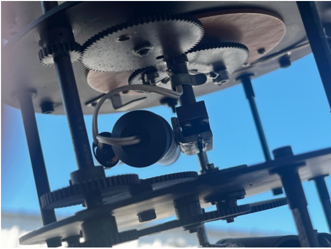
The electrical wiring of planetariums are challenging because it should be able to rotate 360 degrees on each axis. Some contacts like the central filament are powered by a brush + conductive disk method, similar to electric motor armatures.
