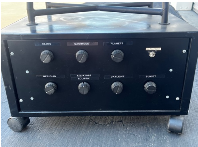
The control panel sets the speed, lamp intensity, sun-set, etc.
