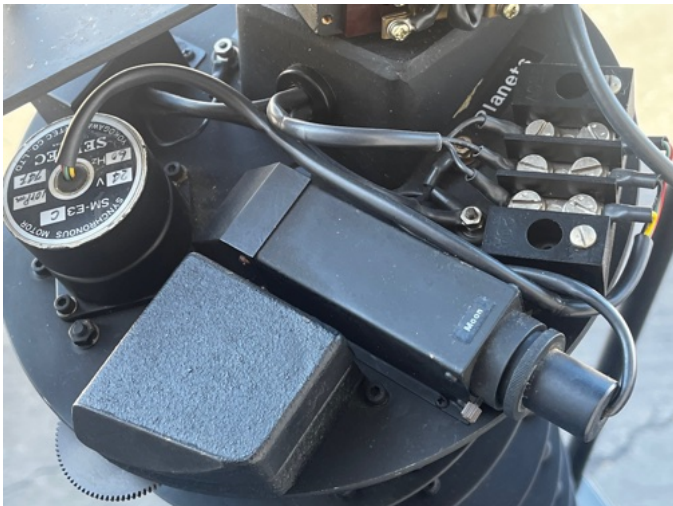
Above left, the main servo drive motor, and the star projector coupling gear (right). There is also a milky way projector that projects the milky way as a fuzzy cloud across the sky (dome).
