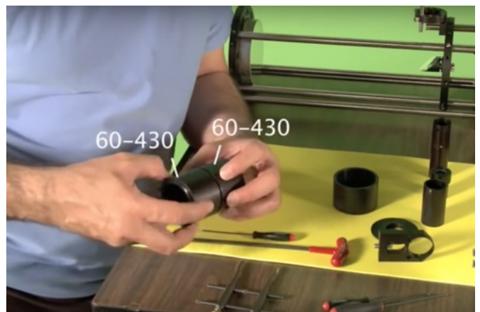
To secure the tubes, the connecting ring is held by nails
