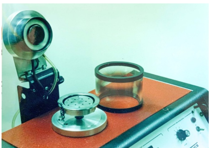
Sputtering Machine lays a thin metal coating on Biological samples.
