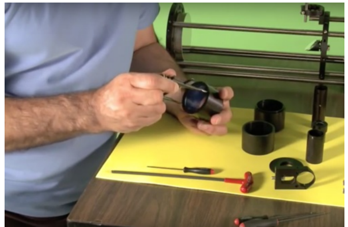
A spanner wrench is needed to secure the rings
