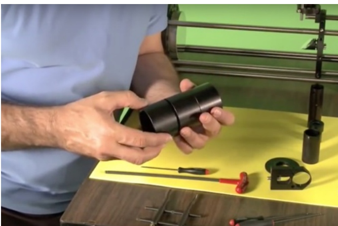
60-430 tubes are added together for the main barrel
